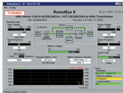
The monitor applet offers real-time analysis of UPS operation.
